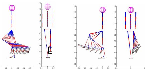
Fig. 5. Humanoid robot stick diagram performing leg bending: a) bending intensity 48%, movement velocity (specified by movement duration) 22% b) bending intensity 46%, movement velocity 74%
